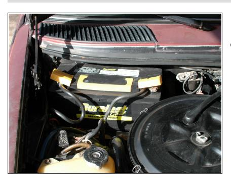
Install the new ground cable, using the new captive bolt, and nut, that came with it. Once you've finished, consider covering the terminal where the cable attaches to the battery in a silicone dielectric grease to prevent corrosion.
