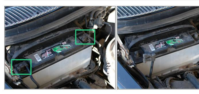
• Start by disconnecting both battery terminals, beginning with the negative (-) side, which travels just a few inches to a bolt attaching the other end to the car's body.
