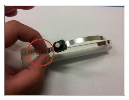
Remove metal apparatus containing button switch first by bending piece in arc shape. Carefully pull out clipped tip as shown.
