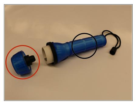
Remove light mechanism from body containing battery. Twist light bulb (red circle) counterclockwise while holding base of flashlight (black circle).
