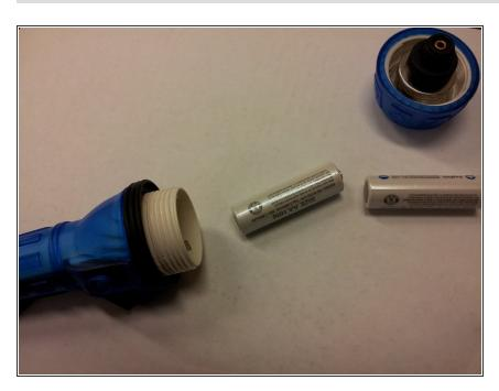
Angle body of flashlight until two AA batteries fall out. Store battery components.
