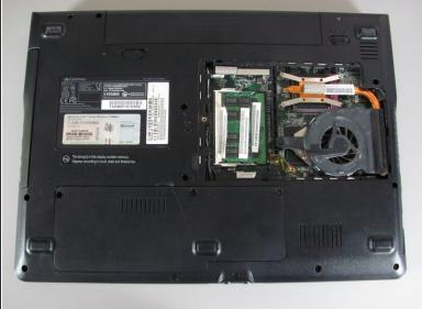
Lift and remove the cover using the spudger.
