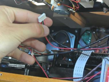
Remove the red and black connection underneath the turntable.
