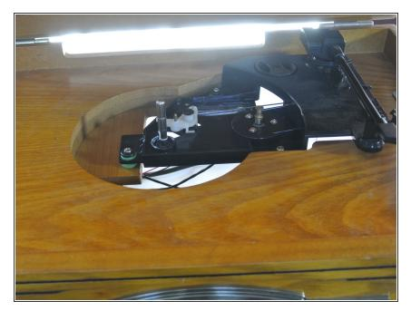
Position yourself in front of the turntable to unscrew the three bushing bolts.
