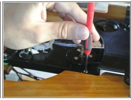
Unscrew the three bushing bolts with the Phillips screw driver.
