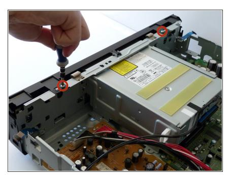
Now, on the front panel, you will want to remove the two 10mm screws on top of the device.
