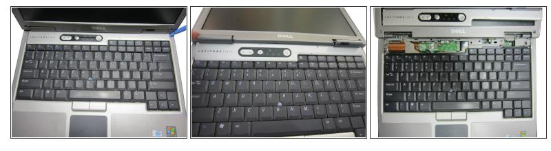
Use an opening tool or flat tool to remove the plastic cover above the keyboard.
