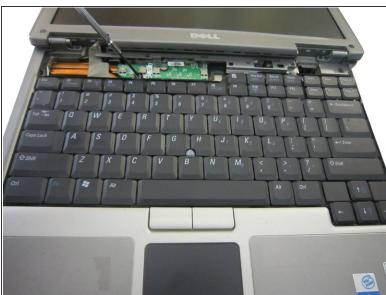
Remove the two 3.9mm Philips #1 screws that are holding the keyboard in place.
