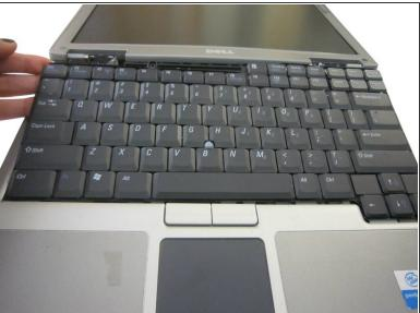
Using an opening tool, carefully release the keyboard from the case.
