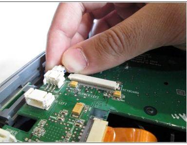
Hold down the release tabs to remove the cables from the white tabs.
