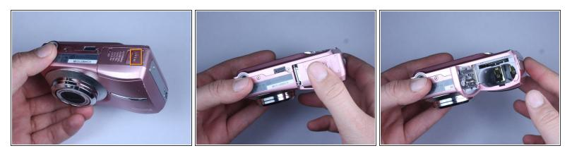
Locate battery compartment on bottom of camera and slide open by applying pressure in the direction of the arrow.
