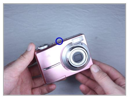
Turn off camera by firmly pressing the power button that is located on the top of the camera near the mode selector dial.
