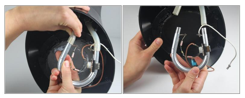
• Separate the tubing from the heating coil by grasping the tubing in one hand and the heating coil in the other. Gently pull them apart.
