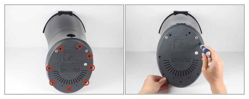
Remove the eight 11 mm screws that secure the base of the machine with a Phillips Head #2 screwdriver.
