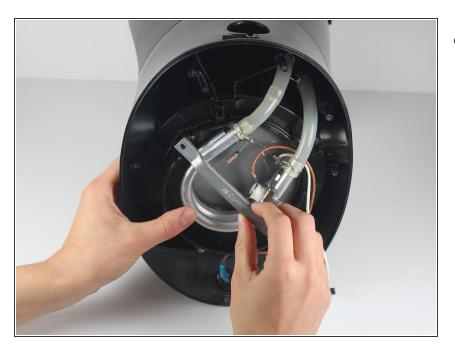
Gently lift the silver support bracket to free the heating plate from the heating coil.
