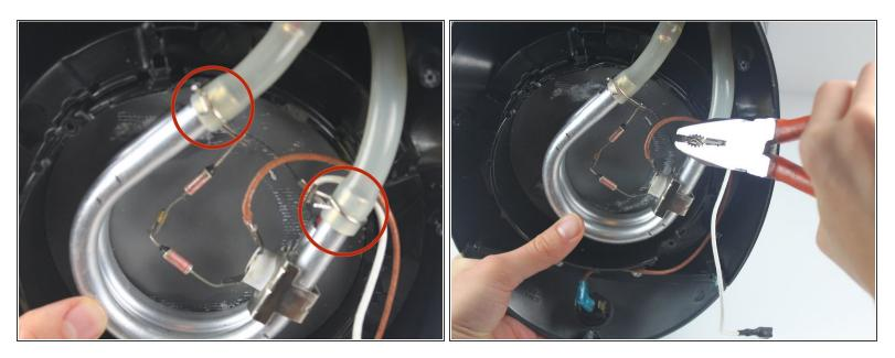
Pinch and loosen the crimps with the needle-nose pliers.
