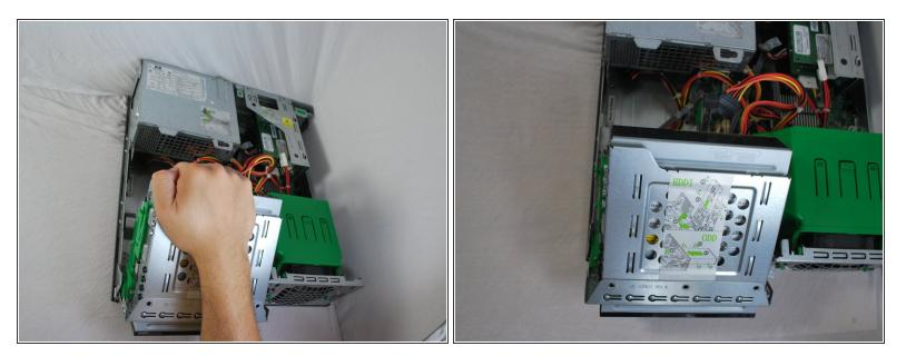
• Using your hand, grip the Optical Drive and lift it up into a 45 degree angle.
