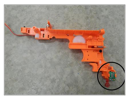
Once you have the handle disassembled locate the triggering circuit board.
