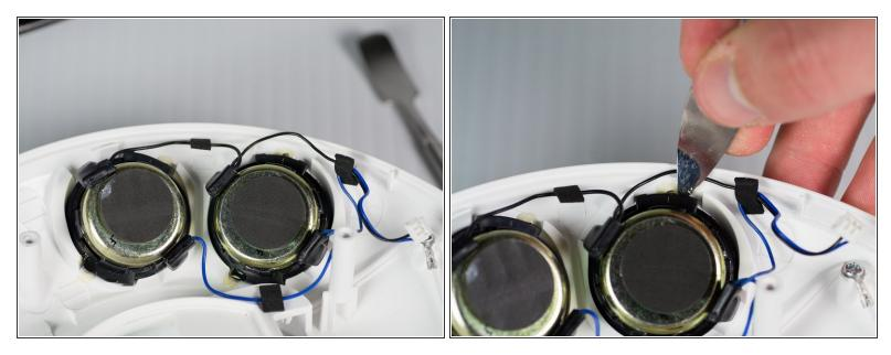
Separate speakers from their slots using a metal spudger.
