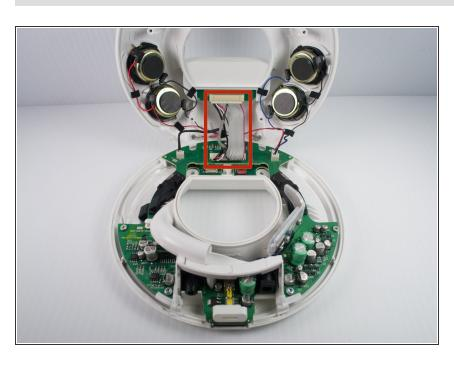
Disconnect the ribbon cable connector from the top half of the device by pulling outward and parallel to the connecting pins.
