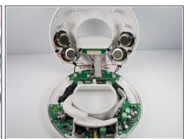
Open the device along its seam.
