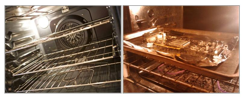
Prevent the GPU components from touching any surface by elevating the edges of the card with foil.
