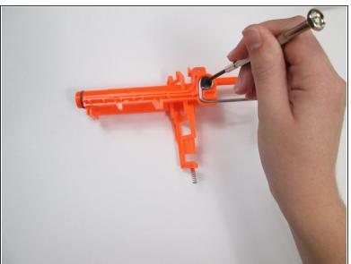
With the hammer rod side of the bullet chamber facing you, unscrew the 5 mm phillips screw holding the hammer rod in place.
