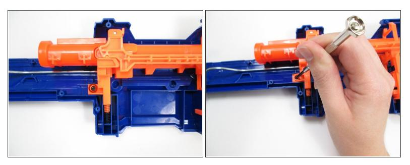
Remove the 5mm phillips screw holding in the chamber lock mechanism.
