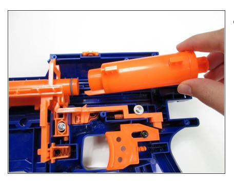
Pull the air cylinder and plunger assembly rearwards and out of the rifle.
