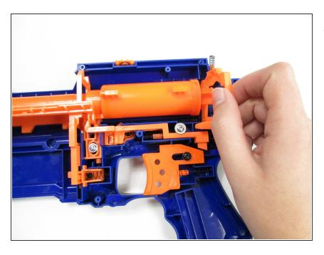
With the plunger in the air cylinder, pull the plunger lock out of the rifle body.
