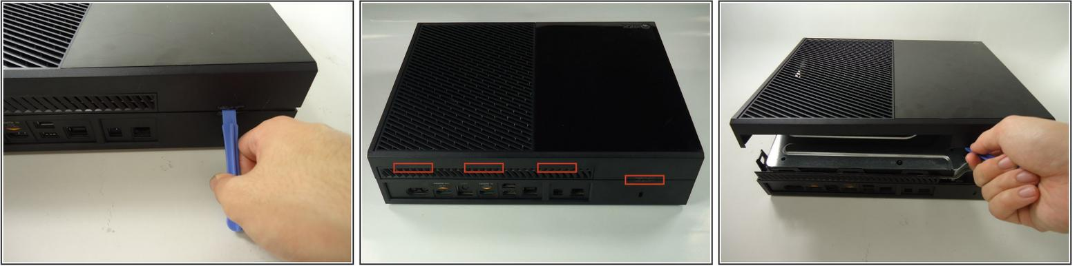
**⚠** Rotate the Xbox and remove the warranty sticker from the back. Removing this seal and opening the case of the Xbox voids your warranty with Microsoft.
