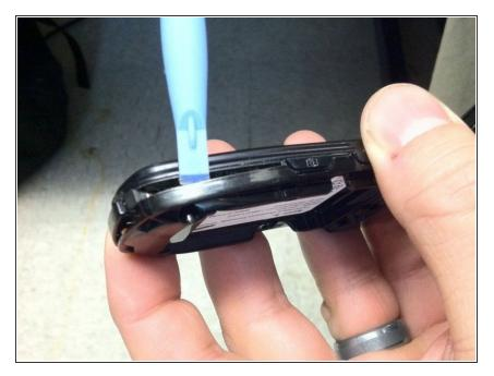
Using spudger, pry off back cover starting at the bottom corners and moving around the perimeter towards the hinge. Disengaging the clips near the hinge may require some force.
