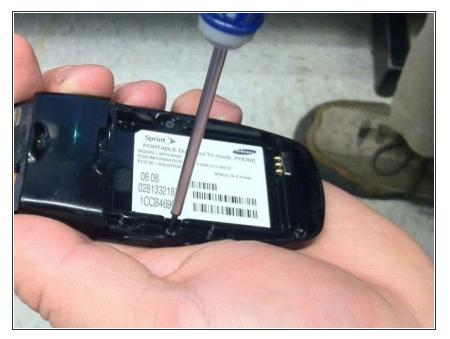
Using a #00 Phillips screwdriver, remove four screws from the bottom half of the phone in the battery compartment. Place screws off to the side.
