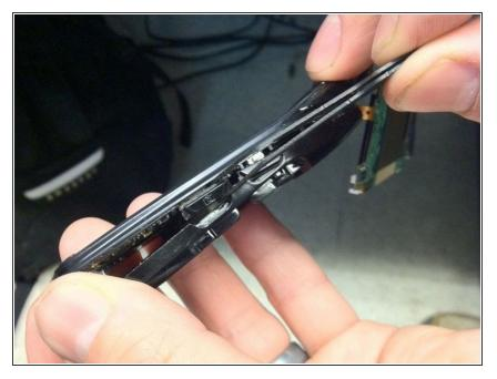
• Using tweezers, carefully remove buttons from both sides while removing back cover. Note the positions of the buttons. They must be returned to the proper positions.
