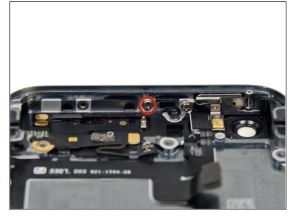
Remove the 1.3 mm Phillips #000 screw securing the logic board grounding bracket to the rear case.
