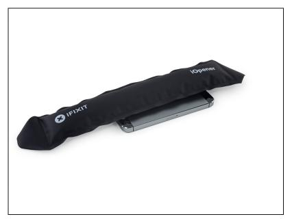
If any of the adhesive strips broke off and the battery remains stuck to the rear case, prepare an iOpener or use a hair dryer to heat the rear case directly behind the battery.
