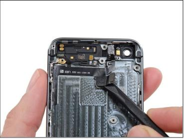
• Slide the flat end of a spudger under the upper component assembly cable to free it from the rear case.
