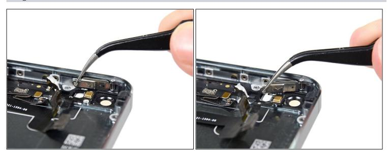
• Use a set of <u>tweezers</u> to swing the power/sleep button bracket away from the case.
