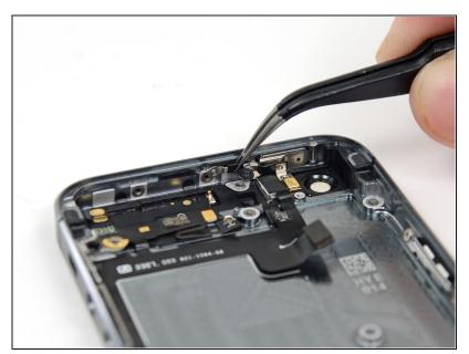
• Remove the logic board grounding bracket.
