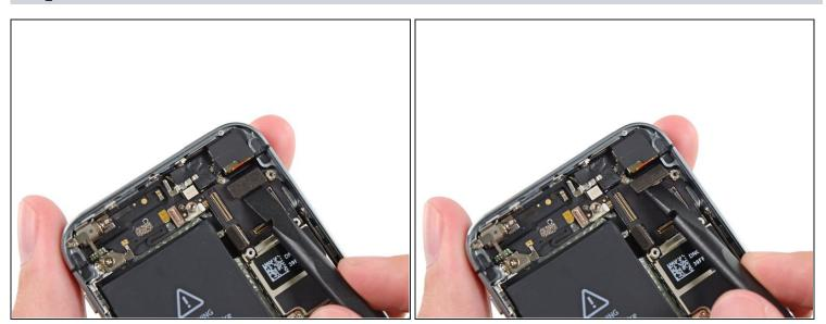
• Use the flat end of a spudger to disconnect the rear-facing camera cable from its socket on the logic board.
