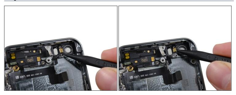
• Use the tip of a spudger to free the microphone portion of the assembly from the case.
