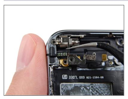
• With a set of <u>tweezers</u>, remove the vibrator bracket.
