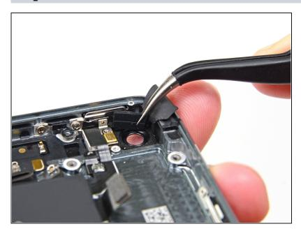
• Remove the rubber camera bumper from the case.
