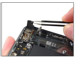
Using a pair of <u>tweezers</u>, flip the rubber camera cover out of its clip and toward the outside of the rear case.
