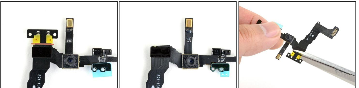
ⓘ If your replacement sensor cable has an extra tab, you'll need to carefully cut it off. You won't need this tab—it's used for parts testing.
