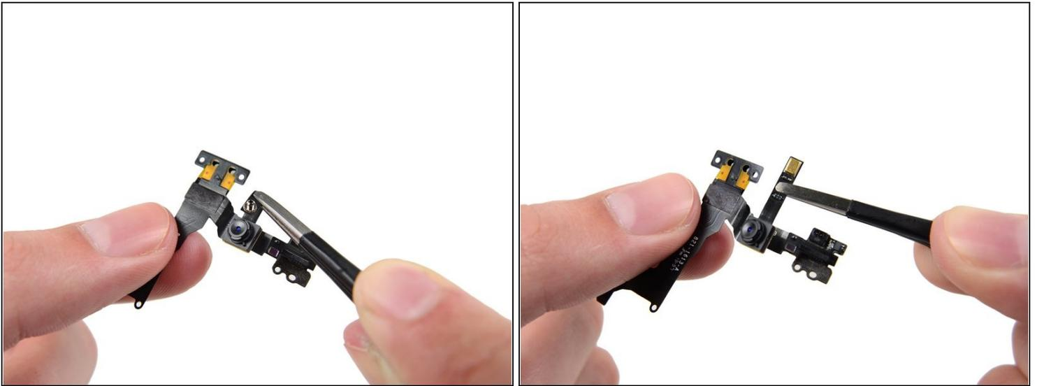
ⓘ In order to ensure a good fit and proper placement of components, make sure your new cable assembly matches the one that came out of your iPhone.
