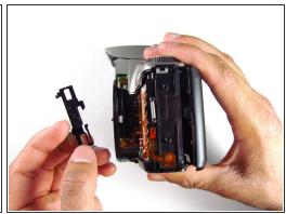
Pull off the lever by pushing up from the bottom and pulling away from the bottom.
