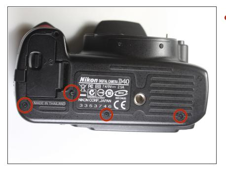
Remove the four highlighted 3.0 mm
