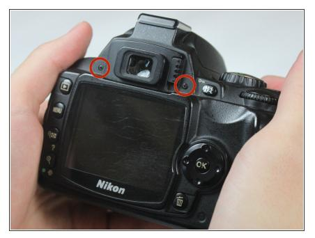
Remove the two visible 6.0 mm
