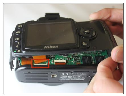
• While pulling the bottom down, remove the back of the camera.
