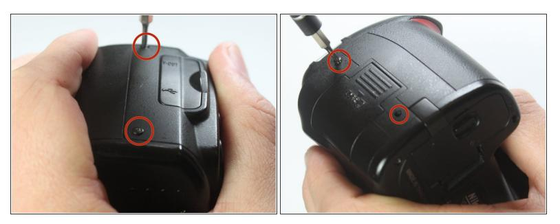
• Remove the four 6.0 mm Philips #0 screws on the left and right sides of the camera.
