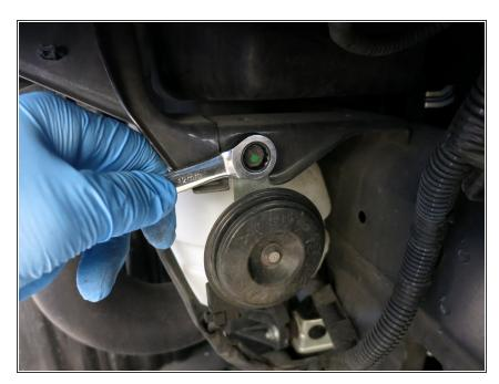
Use a 12 mm wrench to remove the bolt holding the horn in place.
