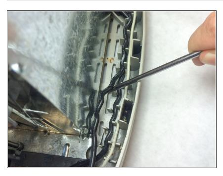
Using a flat-head screwdriver, pry the power cord from the base of the toaster.
