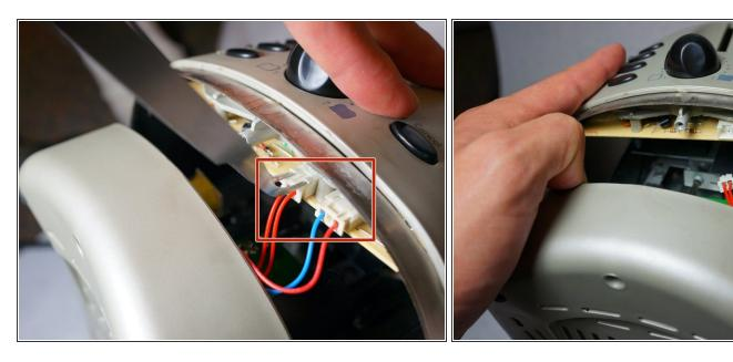
Disconnect the cable clips from the circuit board using the tweezers to free the outer metal shell from the plastic base.
