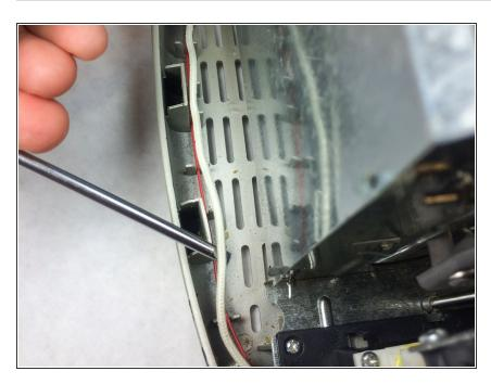
Using a flat-head screwdriver, pry the white wire from the base.
