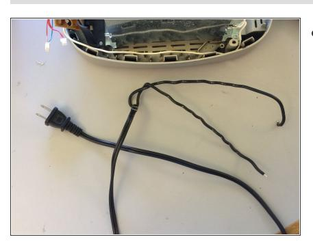
Pull the cord from the base to remove the cable.
