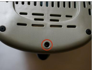
• Using the Phillips-head #2 screwdriver, unscrew the three 1cm Phillips-head screws on the plastic base of the toaster to separate the outer metal shell from the plastic base.
