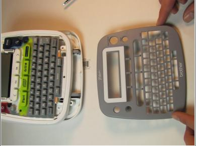
Pull the clips inward two at a time, first the top then the bottom, to snap the face plate off.
