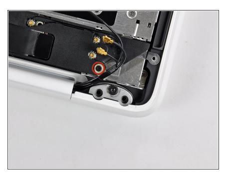
Remove the single 3 mm Phillips screw securing the antenna ground straps to the rear speaker housing.
