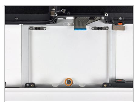
Remove the 1 mm T6 Torx set screw near the front edge of the upper case.
