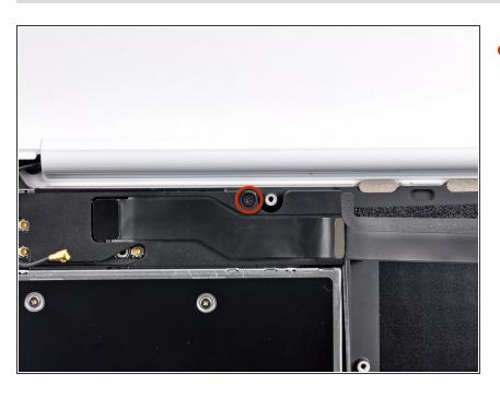
Remove the single 12 mm Phillips screw securing the rear speaker to the upper case.
