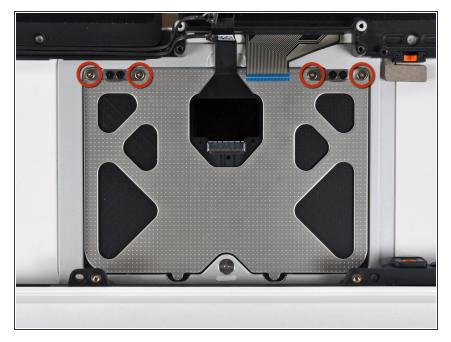
Remove the four 1.3 mm Phillips screws securing the upper edge of the trackpad to the upper case.
