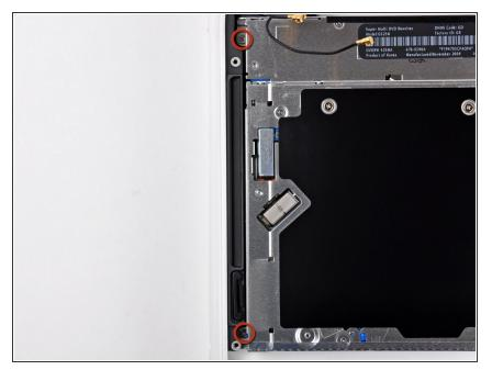
Remove the two 2.5 mm Phillips screws securing the optical drive to the upper case near the optical drive opening.
