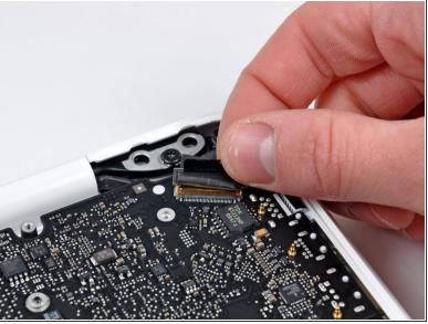
Grab the plastic pull tab secured to the display data cable lock and rotate it toward the DC-In side of the computer.
