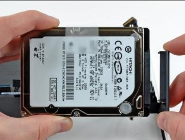
Disconnect the hard drive by pulling the hard drive cable connector away from its socket on the hard drive.
