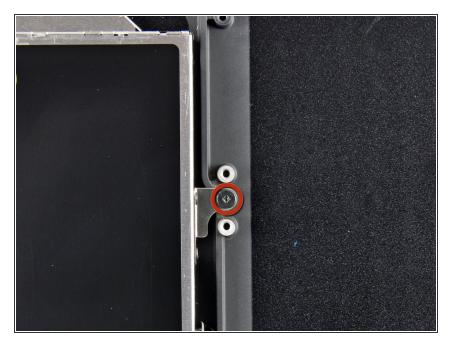
Remove the single 4.5 mm Phillips screw securing the inner edge of the optical drive to the upper case.
