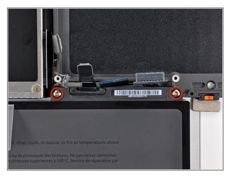
Remove two 5 mm Tri-Wing screws securing the battery to the upper case near the battery connector.
