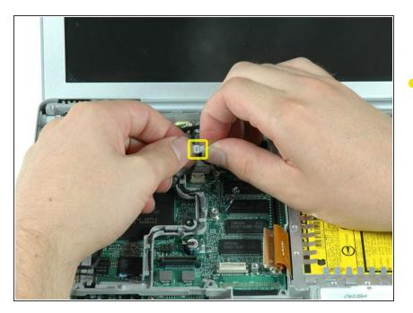
Lift up middle speaker cable from the lower left corner of the fan, and disconnect the two sections of the cable.
