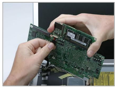
Disconnect the DC-In connector from the underside of the logic board.
