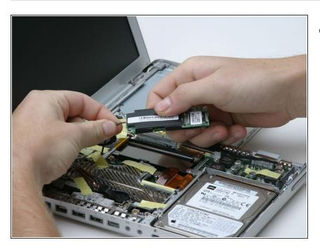
Disconnect the modem cable from the modem.
