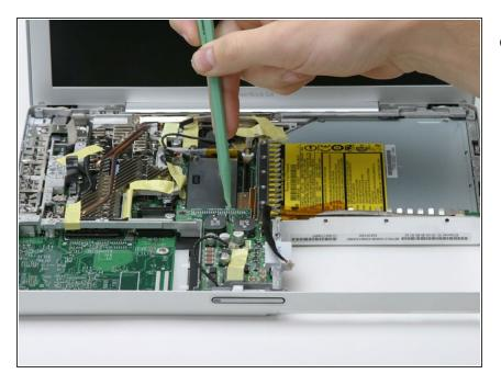
Lift the end of the DC-to-DC board closest to the display and pull the board out of the computer.
