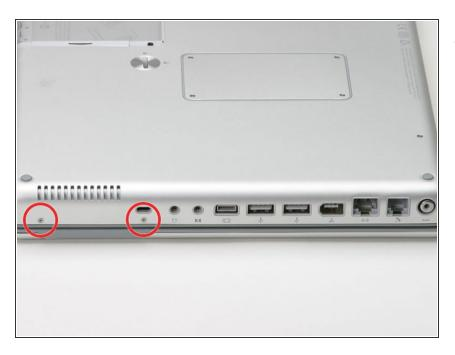
Turn the computer 90 degrees clockwise and remove the two medium-length Phillips screws from the casing.
