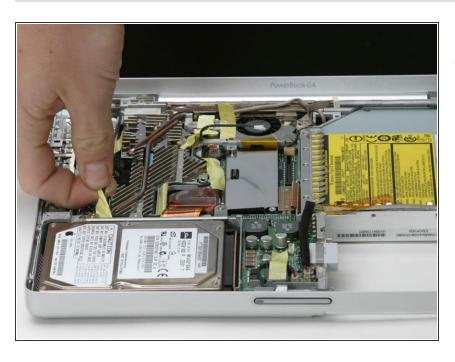
Remove the yellow tape to free the cable from the left side of the heat sink.
