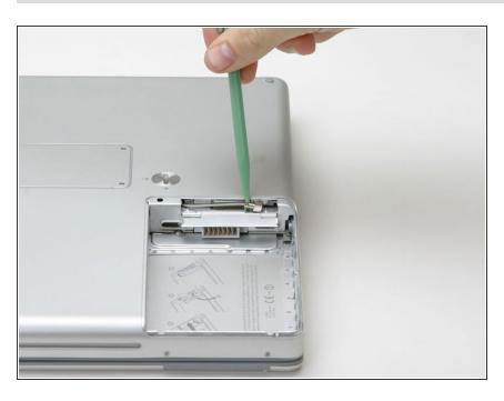
Use a spudger to disconnect the Airport antenna from the card.
