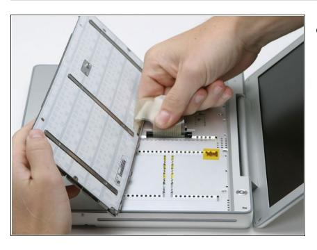
Grasp the keyboard connector ribbon near the connector and disconnect it from the logic board.
