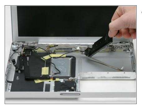
Slide the subwoofer away from the screen and out of the computer.
