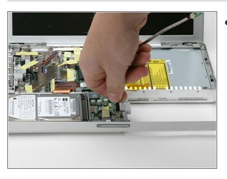
Disconnect the reed switch cable from the DC-to-DC board.
