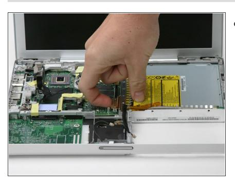
Disconnect the orange optical drive cable from the logic board.
