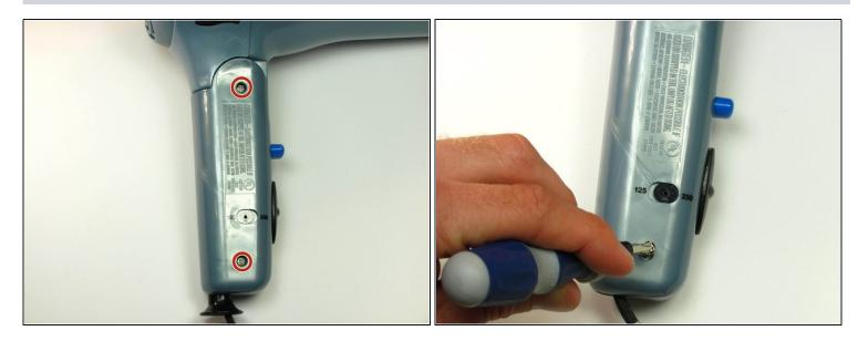
Unscrew the two 18 mm long Phillips #2 screws on the side of the hair dryer.
