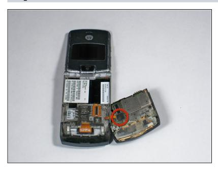
Peel off the connector between the motherboard and the body of the phone.
