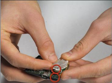
• Pull out the white plastic cover by unclipping the two plastic pieces shown.
