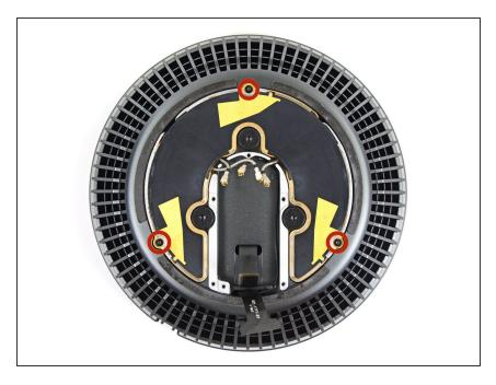
Remove the three 3.7 mm T4 screws securing the antenna array to the fan assembly.
