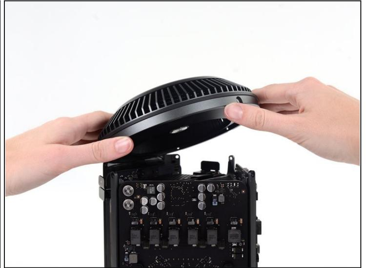
ⓘ The fan assembly is attached to the rest of the computer by two cables on the IO board side.
