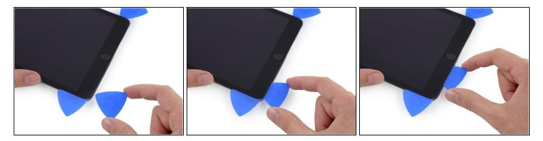
(i) Leave the pick from the last step in place to prevent the adhesive from re-sealing.
