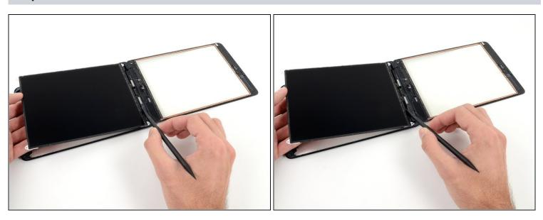
(i) Two wide strips of tape connect the LCD to the speakers.
