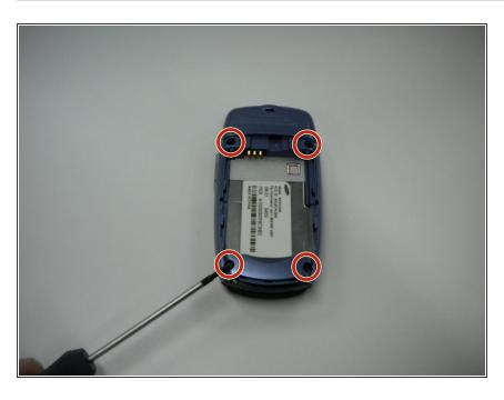
The lower casing is held on by four screws in the corner of the battery enclosure. Remove these screws.
