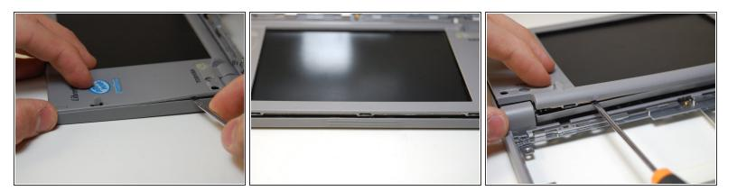
• With a spudger or a flat screwdriver open the screen as shown.
