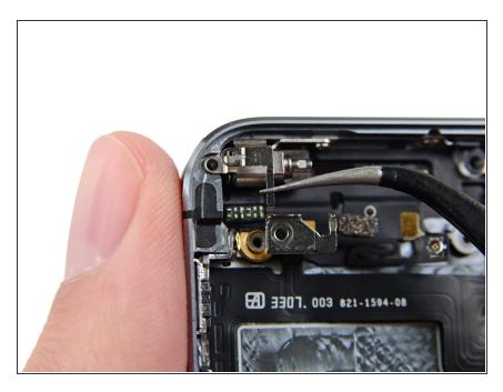
With a set of tweezers, remove the vibrator bracket.
