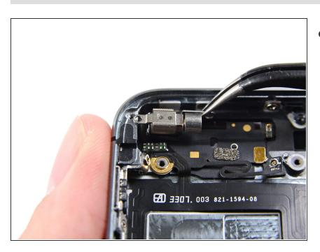
Use a set of tweezers to remove the vibrator from the rear case.
