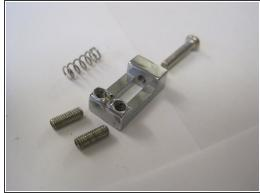
Undo the 6 screws holding the saddles to the bridge. Then remove the spring and unscrew the 12 threaded bars.
