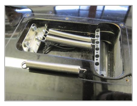
Remove the three tremolo springs from the spring claw and tremolo block.
