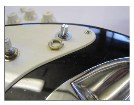
Unscrew the three bolts holding the tone/volume potentiometers to the scratch plate.
