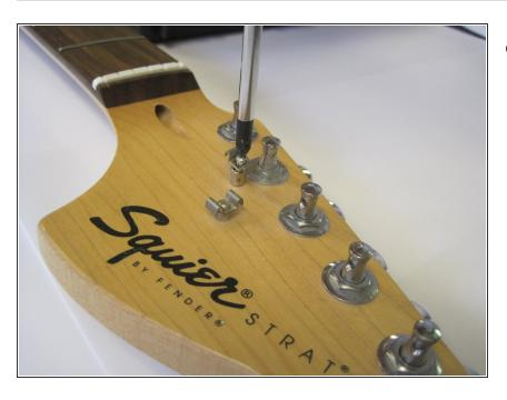
Unscrew the two small screws securing the string trees to the headstock.
