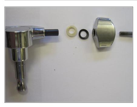
Remove the tension screw followed by the tuner button, metal and then fiber washer.
