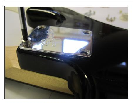
Remove the four wood screws holding the neck to the body of the guitar.
