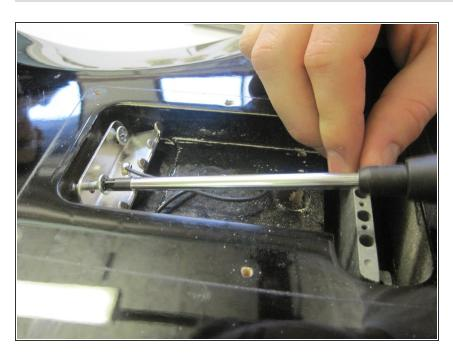
Unscrew the two screws holding the spring claw to the body.
