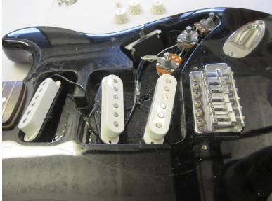
• Lift off the scratch plate, revealing the electronics inside the main body
