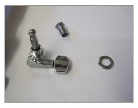
Push the tuners from the front to pop them loose. It make take a bit of force if the alignment peg is stuck.
