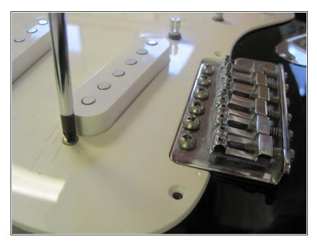
unscrew the six screws holding the three pickups in place.
