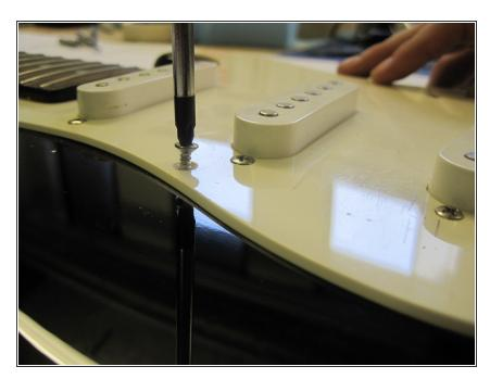
Unscrew the eight screws which hold the pick guard to the main body.
