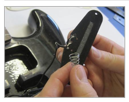
Remove the springs which were on the underside of the pickups.
