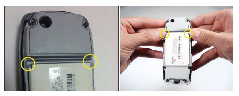
• To release the battery, press the two tabs that are located directly above the battery towards the top of the phone at the same time.
