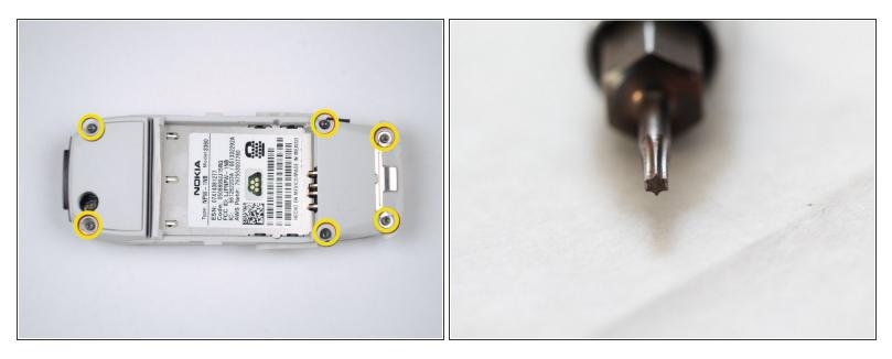
Remove the six screws using a T6 screwdriver. (refer to second picture to help identify T6 screwdriver head).
