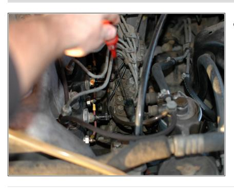
Return the dipstick to the tube when completed and be sure to push it all the way in until it seats properly in the tip of the tube.
