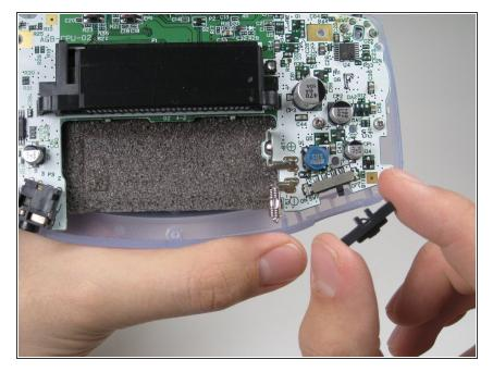
Remove the gray On/Off Switch by pulling up and away from the unit.
