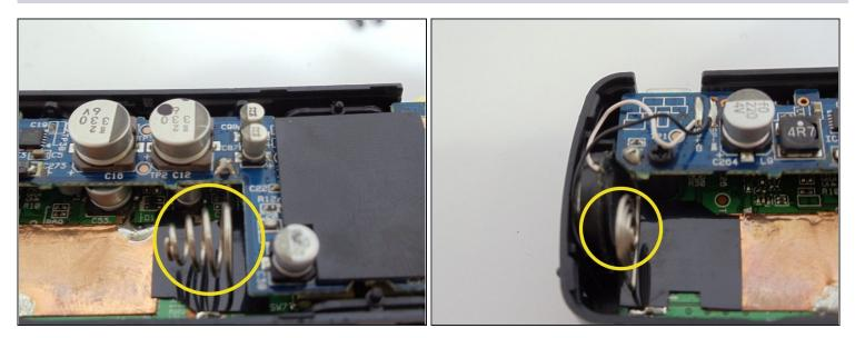
• Remove the faulty terminals
