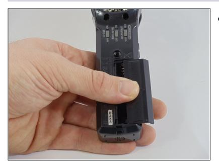
• Remove the battery cover, pressing down on the tabs and sliding.
