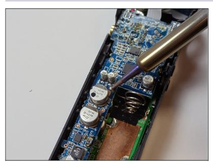
• Place new lead in at point one and re-solder at the point.
