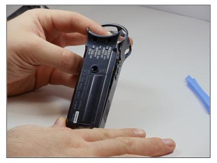
• Carefully pry up the top end of the back cover using one finger
