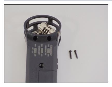
• Unscrew the two (2) #00, 10 mm screws located below the mic on the back cover
