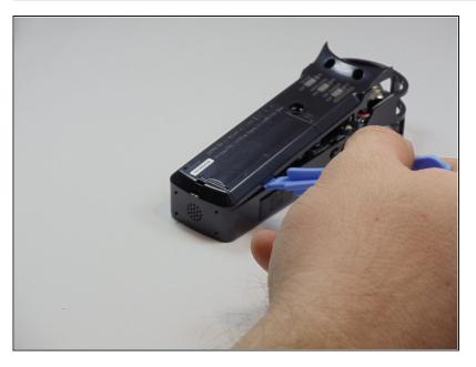
• Remove the back plate by using a plastic removal tool to pry the back cover up around the edges.
