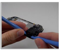
• Use a plastic opening tool to remove each area holding the parts together.
