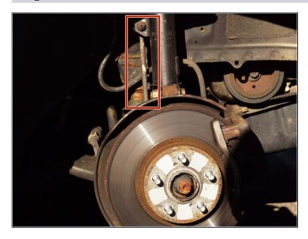
The sway bar link is located behind the brake shield, connecting the sway bar and suspension.
