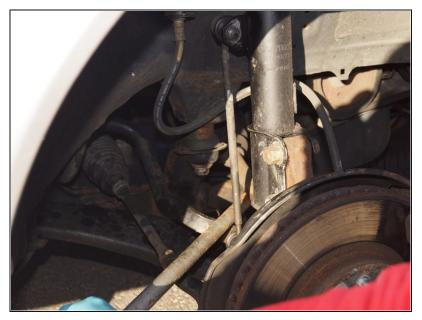
After taking all the nuts off, use the bar from the hydraulic jack to push down the sway bar so that it is easier to take the sway bar link off.
