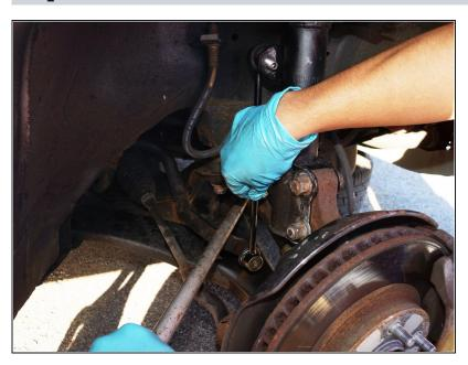
To put the new sway bar link in, use the bar from the hydraulic jack to push down the sway bar, and then insert the new sway bar link.
