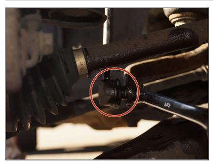
Repeat Step 7 for the bottom nut of the sway bar link.
