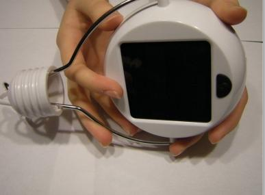
• On the other side, firmly pull outwards on the handle until you can slide it into place.
