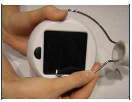
With the handle in one hand and your Nokero Shavano N220 in the other, insert one side of the handle into the hole.
