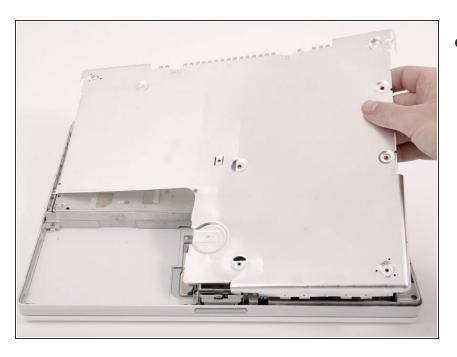
Lift the bottom shield off.
