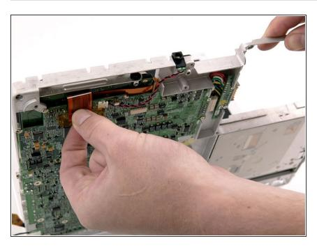
Tilt the computer up and disconnect the orange hard drive ribbon cable from the logic board.
