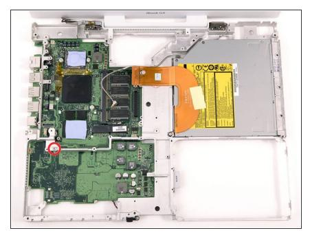
Remove the single Phillips screw securing the logic board to the metal framework.
