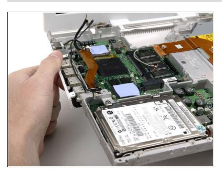
Lift up the left side of the computer and slide the I/O bezel away.
