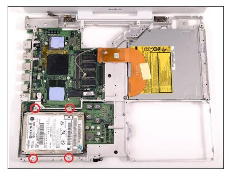
Remove the four Phillips screws securing the hard drive to the metal framework.
