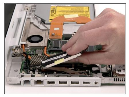
Lift the modem and modem shield from the bottom.
