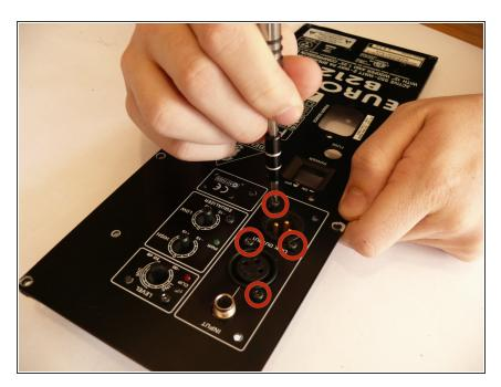
Remove the 4 indicated 9/32" long screws using a #1 phillips head screwdriver.
