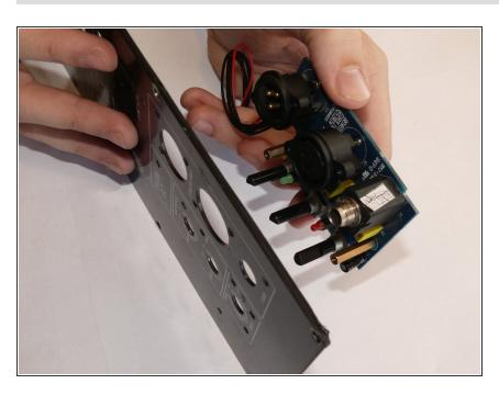
The control PCB is free now, ready to be removed from the speaker's back panel.
