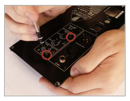
Remove the 2 indicated 3/16" long machine screws with a #1 phillips head screwdriver.
