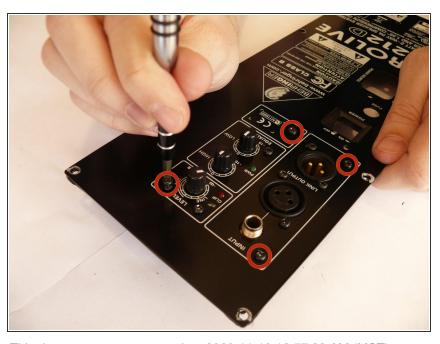
Remove the 4 indicated 9/32" long screws with the #1 phillips head screwdriver
