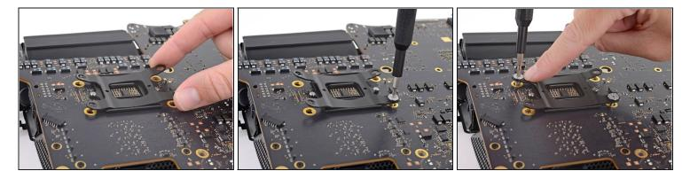
• Place the spring plate on the backing plate.
