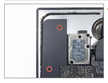
• Remove two 10 mm T10 screws.
