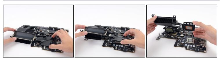
• Lift the heat sink up from the logic board.
