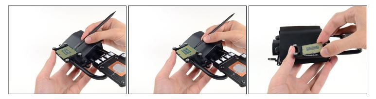
(i) The CPU will most likely be stuck to the heat sink with thermal compound.
