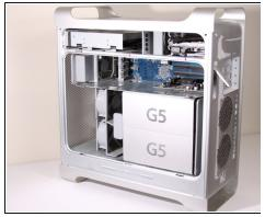
• Remove the air deflector (the clear plastic cover) by pulling on the handle.
