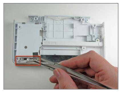
• Carefully use a pair of <u>tweezers</u> to remove the volume switch.
