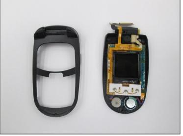
While grasping the top and bottom sections torque the pieces until the indicated hinge has popped out. The two sections of the phone are now able to separate.
