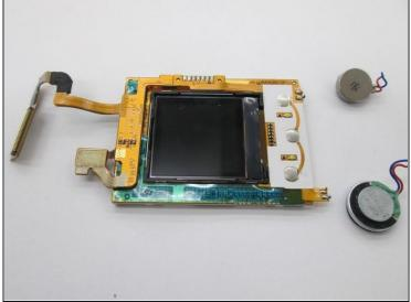
• Use a pair of <u>tweezers</u> to disconnect the speaker wires from the circuit board. Note that the soldered connection must be broken for this to occur.
