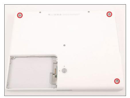
Remove the three newly-revealed Phillips screws.
