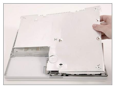
Lift the bottom shield off.
