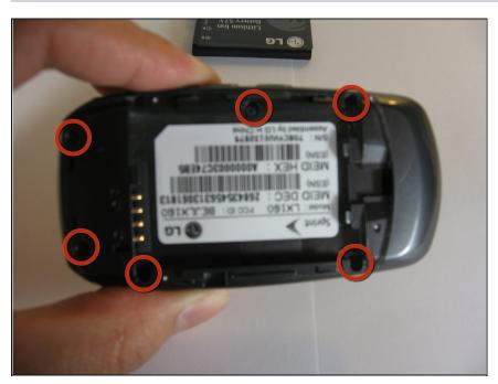
Now turn the phone so that you can see the back where the battery was. Using a screw driver, unscrew the 6 screws holding the back casing together.
