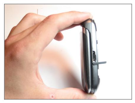
Before continuing pull off all the rubber tabs to the headphones, and the power input.
